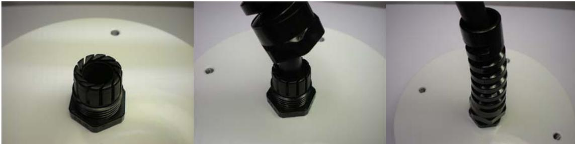
**Bottom Egress Cable Seal** – A water tight integrated cable seal and strain relief was used to seal the cable exit point on the bottom of the camera. A silicone sealant is used to seal the strain relief to metal housing joint. The strain relief provides a water tight seal around the cable itself.
