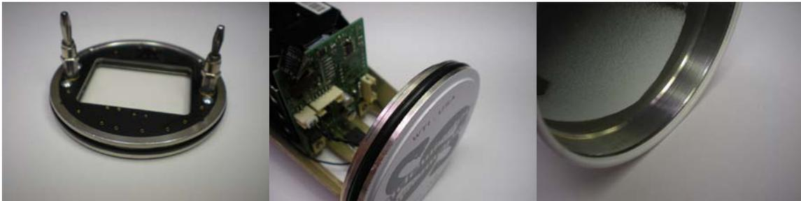
Front and Back Plate to Camera Tube Seal – Sealing the window face plate and the rear plate to the camera housing tube is accomplished using -45C to +120C temperature rated, Shore 65 hardness o-ring seals. The o-rings are greased with a -40C to +95C temperature rated silicone lubricant to provide an air tight and water tight seal. The o-ring seals mate with the precision machined surfaces on the inside front and inside rear of the camera housing tube.
