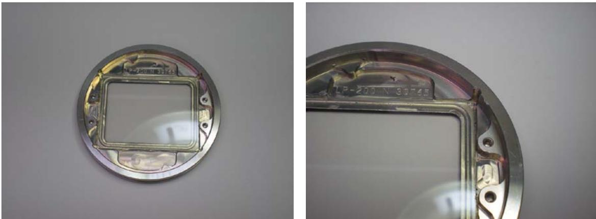
**Window Glass –** Sealing the viewing window glass presents a bit of a challenge, as two materials with different temperature coefficients of expansion must be joined together. A silicone adhesive with a moderate Shore A hardness of 30 and a -60C
