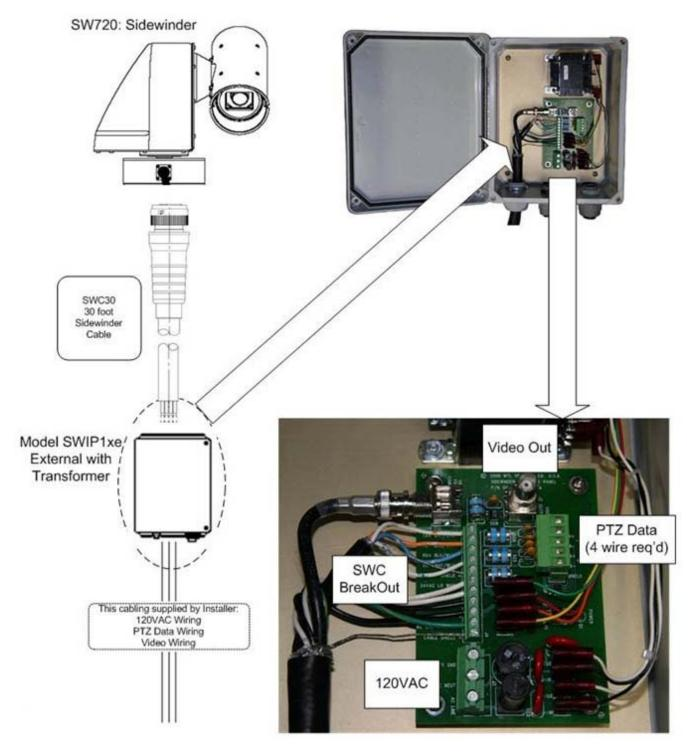
NOTE: The interface panel is required for all Sidewinder camera installations.
