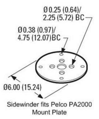
NOTE: The Sidewinder requires mounting in vertical orientation with camera head at top. Please specify which mount you require when ordering your Sidewinder.
