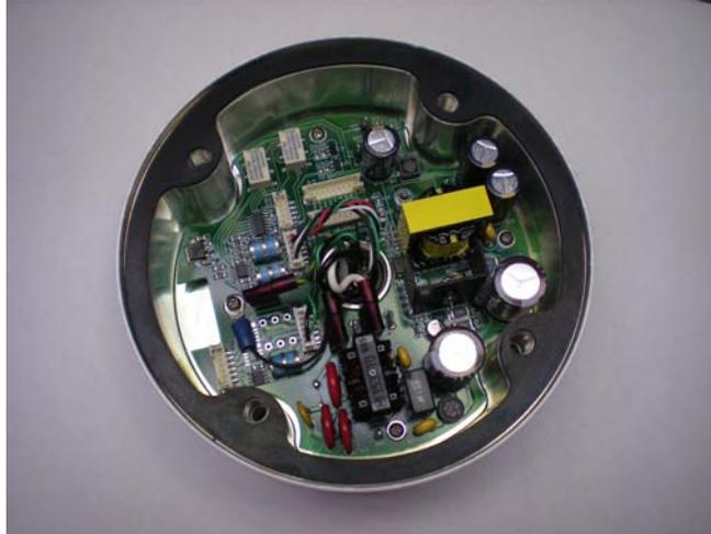
**Power Supply Base Seal** – The power supply base seal was actually pretty straight forward to implement. Since the main camera base structure is very heavy duty, large bolts could be used to apply the force necessary to get a highly reliable seal. A special laser cut gasket is used to seal both the mounting rim and the mounting bolts.
